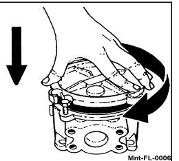
5. Remove filter. Inspect material trapped by the filter. It can indicate parts wear in the system. Mnt-FL-0008
